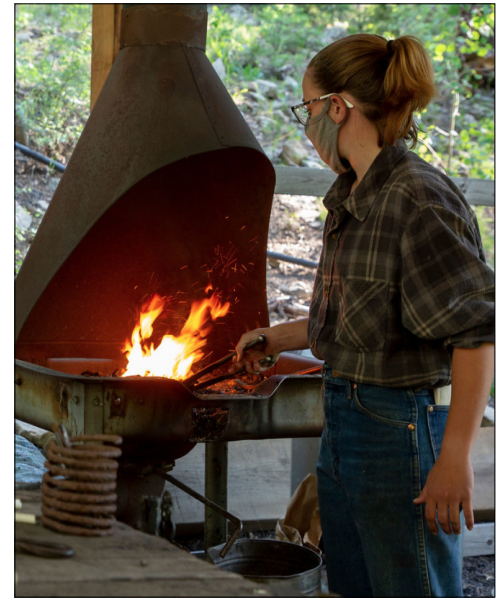
Blacksmith Sydney Marie Bascomb removes a piece of hot steel to be forged by a crew at French Henry.
