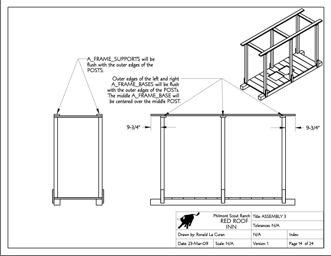
A\_FRAME assemblies are to be spaced in 2ft intervales from the center to center with the two A\_FRAME assemblies on either side of the Red Roof Inn being flush with the ends of the A\_FRAME\_SUPPORTs they are resting on. This will result in there only being a spacing of 22-1/2" between the final two A\_FRAME assemblies on one side.
