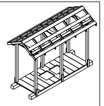
The sides of the two outer ROOF\_SLATS should be flush with the edge and the peak of the A\_FRAME assemblies. The third should be located in between them, roughly 16-1/4" from centerline to centerline of either of the outer ROOF\_SLATS.
