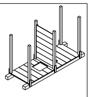
The CENTER\_WALL assembly wil fit exactly between the two center POSTs. It should be placed flush on the floor boards and arrange the wall such that the back sides of the framing on the CENTER\_WALL are flush with one side of the two center POSTS. This will center the CENTER\_WALL adequately.
